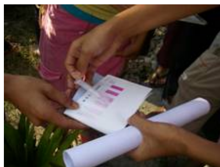
Checking water content by inserting some water in a small tube with Pack Test water quality kit reagent and checking the color after it reacts
